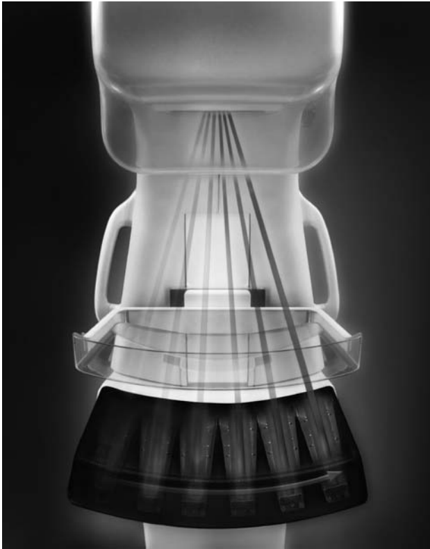
Fig. 4 Principle of the slot-scanning system using a highly collimated fan beam that covers the active area of the detector. Data are acquired by simultaneous scanning of the breast by the X-ray beam and the detector, both attached to a pivoting arm in the gantry of the digital unit. The movement of the detector inside the mammography unit ( front view ) is represented in transparency. Courtesy of Fischer Imaging, France
